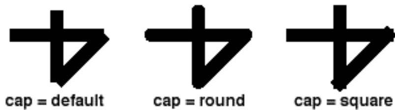
Figure 5: Example of lineMode attribute "cap"
